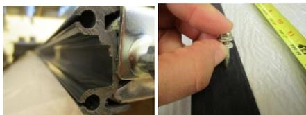
8. Install the weather seal into the bottom retainer by sliding the rubber into the grooves on the bottom panel, the bottom retainer has different sized grooves, be sure the weather seal is slide into the correct holes. The weather strip may stick out from the ends. Cut to 3" past the end and tuck it back into itself, preventing the seal from sliding back or forth.
